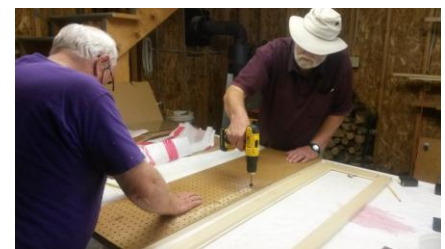
Figure 3drilling holes for shelf pegs, pegboard as our guide for spacing the holes
