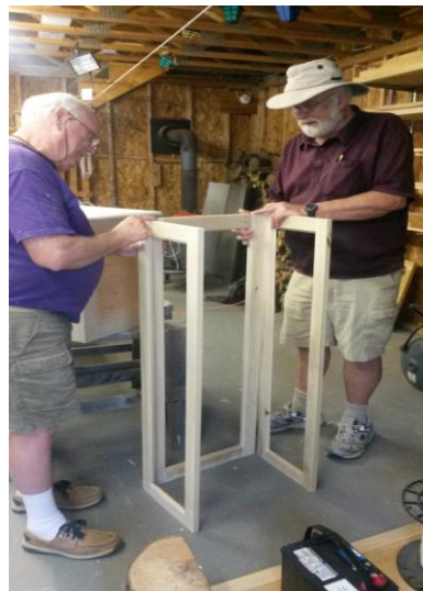
Figure 6 checking to see just how they go together. The panels will have glass sides and front with plywood in the back section.
