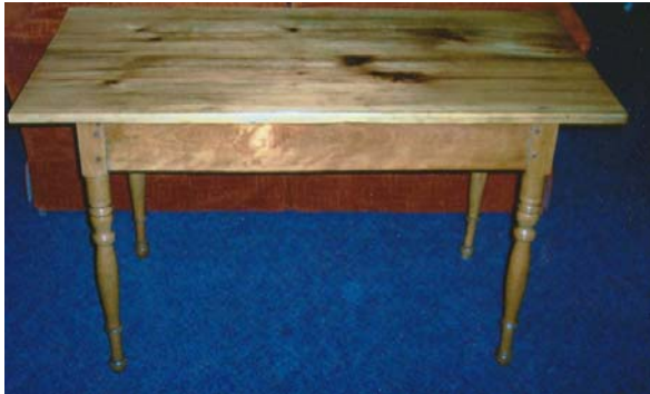
Phil restored this table, mortised and pegged the legs.
